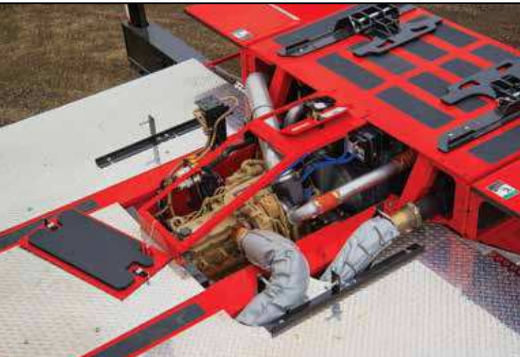
Swing-out doors provide exceptional access to engine components.
