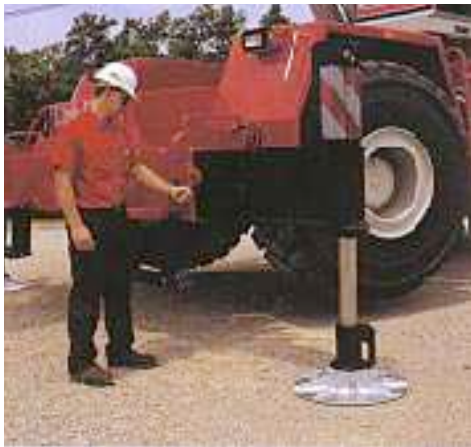
Fully Extended Outriggers 22' 0" (6.71 m) spread
