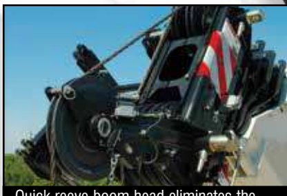
Quick reeve boom head eliminates the need to remove the bucket when it becomes necessary to change the reeving
