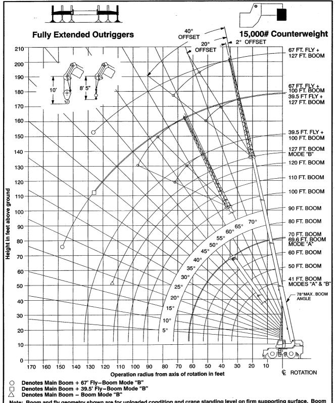
Note: Boom and fly geometry shown are for unloaded condition and crane standing level on firm supporting surface. Boom deflection, subsequent radius and boom angle change must be accounted for when applying load to hook.
