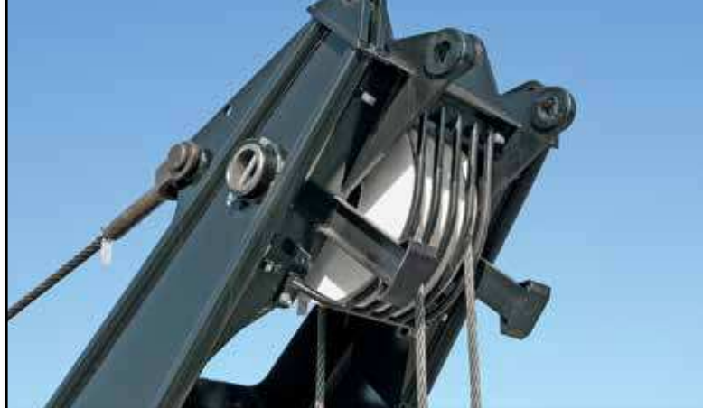
Four polymer head sheaves with maintenance free sealed bearings
