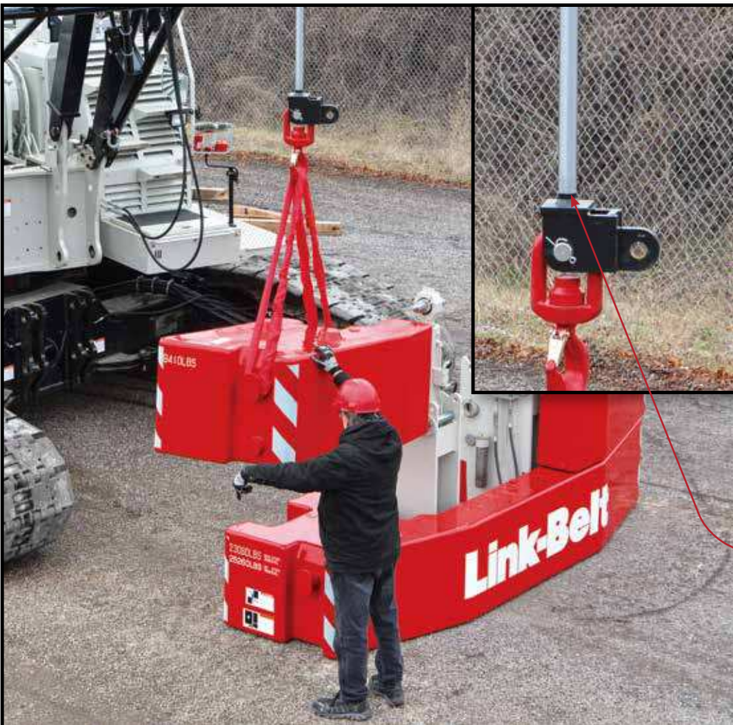
Counterweights lower completely to the ground
