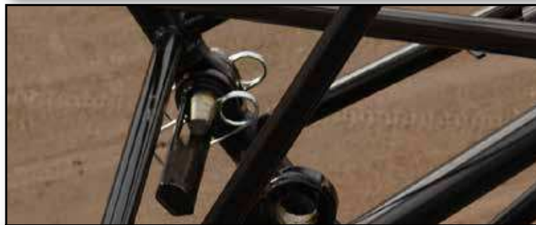
Double tapered connecting pins allow installation/removal from outside of boom. Boom connecting pins store in pin catchers for transport.
