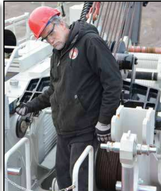
Counterweight removal controls located on work platform at the rear of the crane
