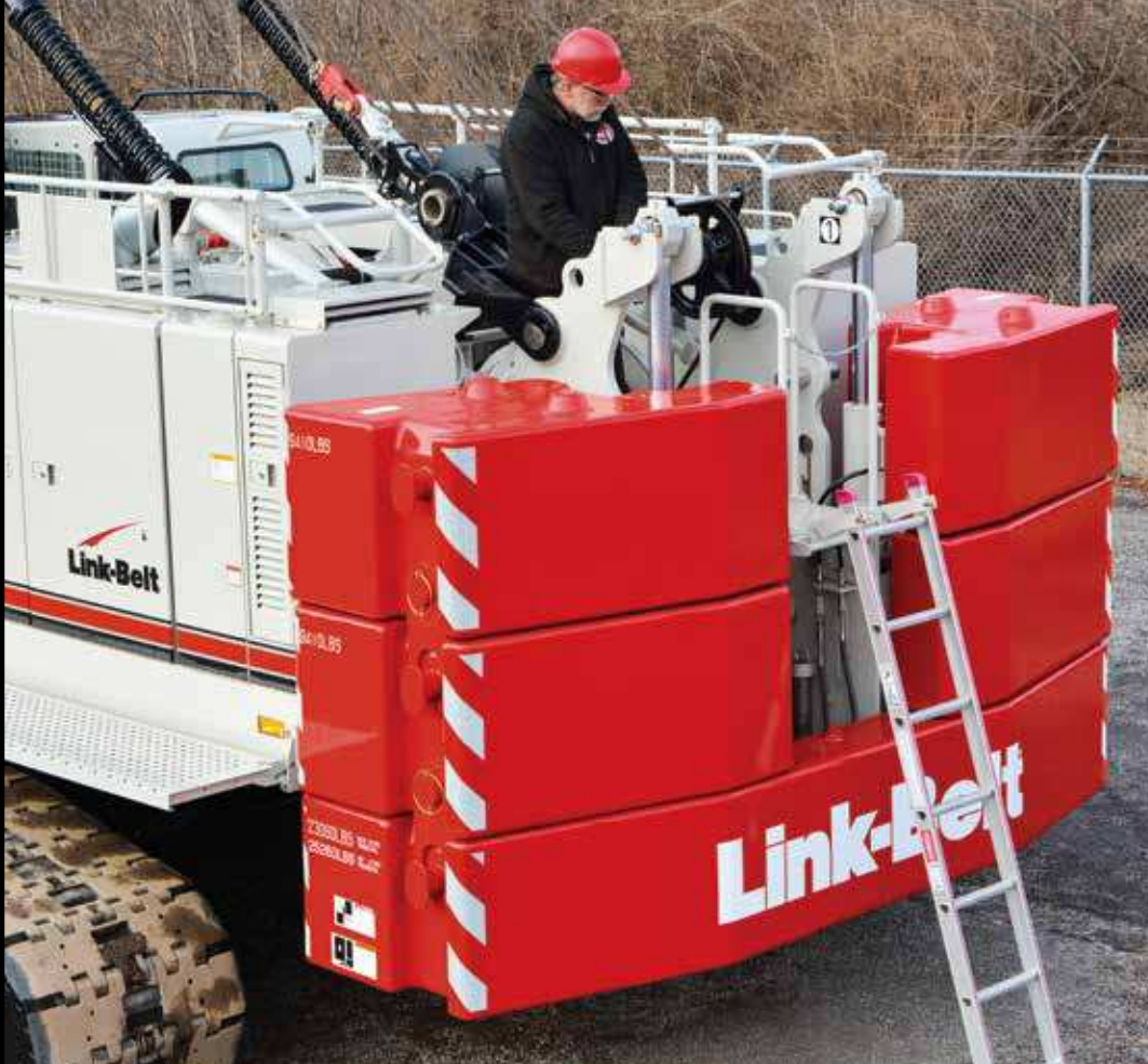
Counterweights lower completely to the ground
