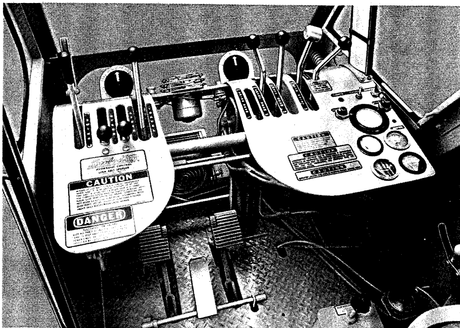
Operator control console
