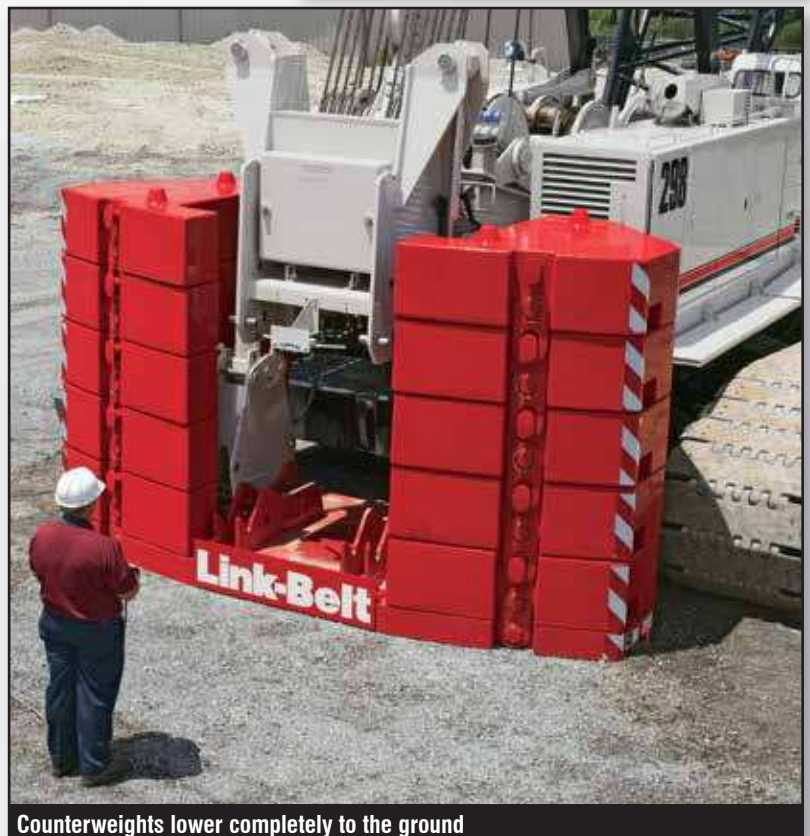
Unlatch cylinders and tray from counterweight than retract cylinders for transport
