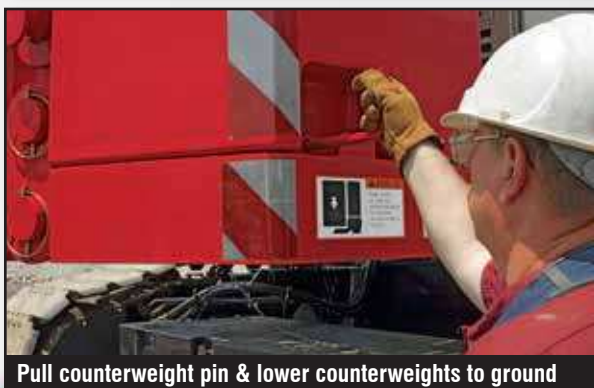
Unlatch cylinders and tray from counterweight than retract cylinders for transport
