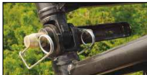
Double-tapered boom pin with pin catcher
