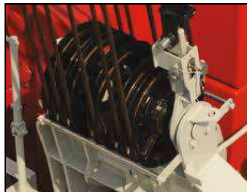
Double-tapered boom pin with pin catcher
