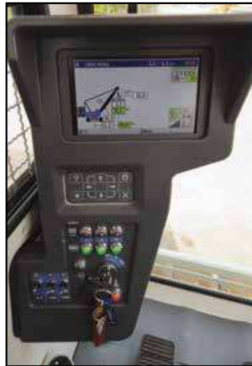
HSL capacity limiter with high visibility color graphic display
