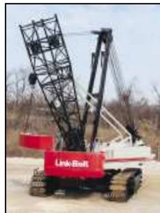
Optional 10' (3.05 m) boom extension handles treads, counterweight and boom during self-stripdown or erection.
