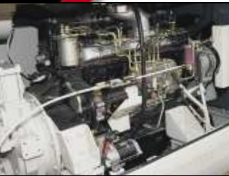
207 hp Isuzu A-6SD1T-QB engine
