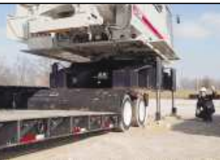
Hydraulic jacking system lifts the upper, lower frame and treads off the ground. Treads are removed and a trailer can then be backed under the lower frame and upper for transport.
