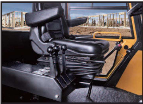
CLOSED CAB: The all-weather closed cab option is equipped with sound insulation, defroster fan, heavy duty heater, ergonomic controls, sliding windows, removable doors, and a 360 degree visibility for safe, efficient operation.
