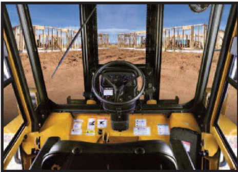
CLOSED CAB: The all-weather closed cab option is equipped with sound insulation, defroster fan, heavy duty heater, ergonomic controls, sliding windows, removable doors, and a 360 degree visibility for safe, efficient operation.
