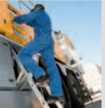
The integrated ladder provides the driver with safe access to the slewing platform and the lift cab.
