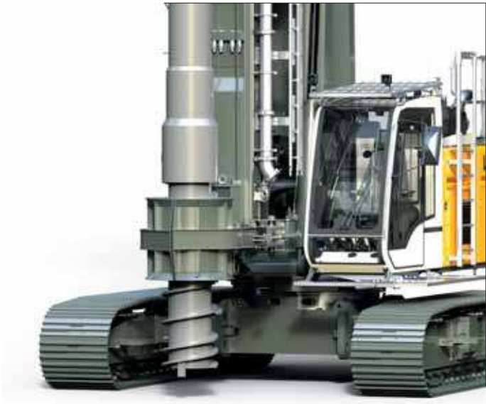
Full displacement tool with auger guide
