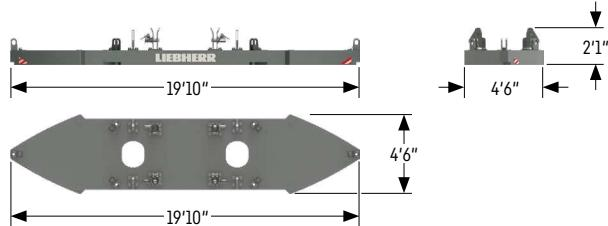
**Basic counterweight slab without tie-down (1x)**
