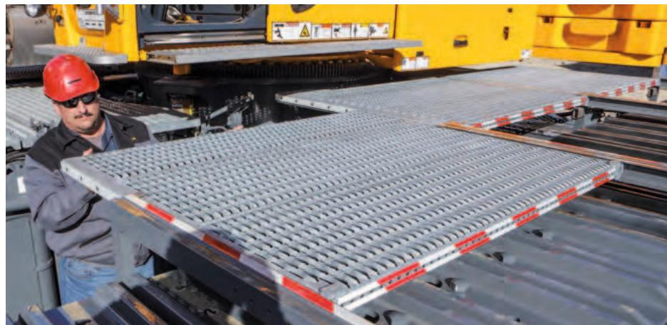
Large grating areas facilitate safe movement on the crane. During the design of the walking areas, special attention was paid to easy and fast transportation and assembly possibilities.
