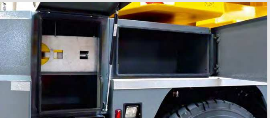
Numerous storage boxes for extensive accessories, lifting tackle and support timber
