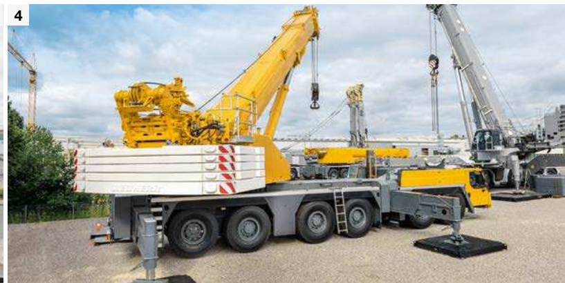
1 Winch 2 secured to the ballast plate 2 Winch 2 is moved hydraulically towards the turntable frame 3 The pulley block is moved towards winch 2 using BTT 4 Winch 2 is installed
