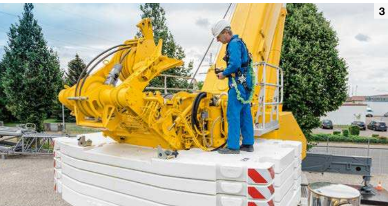
1 Winch 2 secured to the ballast plate 2 Winch 2 is moved hydraulically towards the turntable frame 3 The pulley block is moved towards winch 2 using BTT 4 Winch 2 is installed
