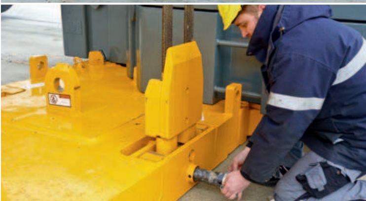
Simple pinning of the base plate to the ballasting device
