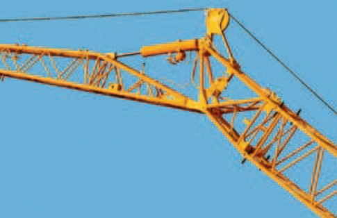
Hydraulically adjustable swing away jib (0° - 40°)
