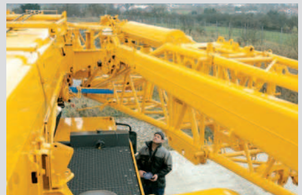
Hydraulic assembly support for attaching the swing away jib by BTT
