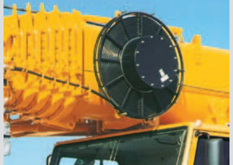
Hose drum for hydraulic cylinder
