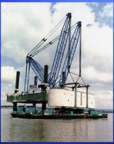
The Lampson Transi-Lift® LTL-1500 is one of the world's most versatile Heavy Lift Crawler Cranes. The Transi-Lift® system is a patented configuration that combines the heavy lifting capabilities of stiff leg derricks and ring mounted lift equipment with the mobility of a conventional crawler crane.
