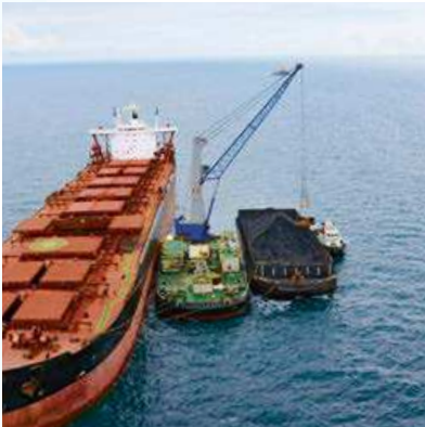
For limited and missing quay infrastructures Konecranes offers floating cranes.
