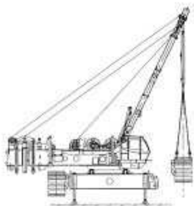
Install the crawler
