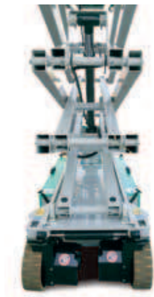
New design of the chassis which allows easy cleaning and ensures protection to the components
