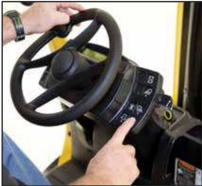
Infinitely adjustable steer column
