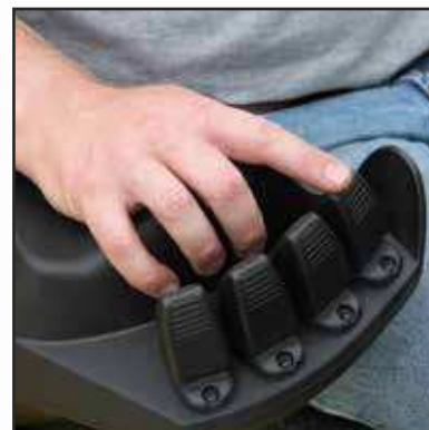
TouchPoint mini-lever electro-hydraulic controls
