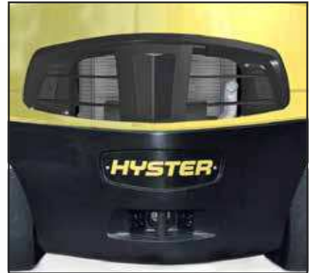
Counterweight venting improves airflow
