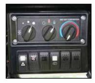
Standard cab heater (air conditioning system is optional). Controls within easy reach of operator's seat.
