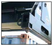
Automatic pendular floating twistlocks with override function; integral carriage with +/-30" sideshift.
