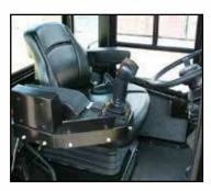
with retractable seat belt for maximum comfort. Reduces vibration and operator fatigue.
