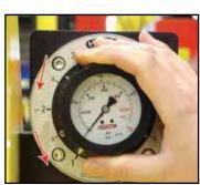
Diagnostic multi-gauge eliminates the need to tap into hydraulic lines
