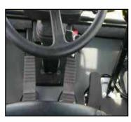
Dual brake pedals - left for brake and declutch, and the right for brake only.
