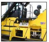
Separate battery cabinet with power disconnect. Separate filter cabinet provides one central location to make for ease of preventative maintenance.
