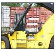
Independently powered traversing cab moves operator forward/backward for optimal visibility and service access.
