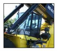
Isolated rubber mounts between cab and chassis, as well as an insulated cab provide a smooth ride and reduced noise levels.
