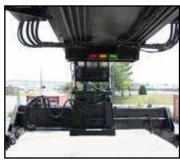
Twistlock engagement indicator lights on boom, as well as inside operator's cab. Interlock safety system ensures proper locking sequence and includes an overload warning alert.
