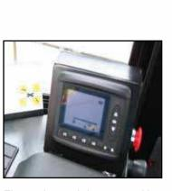
Electronic push-button parking brake control and easily accessible emergency shutdown switch.
