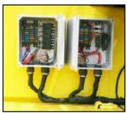
Outboard weatherproof electrical enclosures for easy access and diagnostics.
