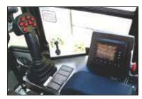
Most ergonomic adjustable armrest with fully integrated hydraulic controls and operator interface. Able to conform to many different body types for unparalleled comfort while operating.
