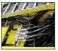
Front removable covers and rear hinged hood on gas struts provide easy access to the entire drive line.
