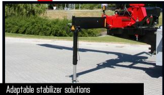
The stabilizer legs of the crane are to ensure stability - however they still have to be sturdy, easy to handle and must not take up too much space when not in use. Therefore you can choose between fixed stabilizer legs, manual swing-up stabilizer legs to 30/60° or manual swing-up stabilizer legs to 180° with gas spring. Stabilizer beams can be freely selected as hydraulically extensible or manually extensible, also in connection with the sophisticated EVS stability monitoring.
