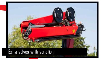
A well-known and usual hose routing to the end of the extensions means that 1 or 2 extra valves are fed in sturdy hose guides alongside the jib extension system. If further efficient protection of the hoses is required, 1 or 2 extra valves can be fed in internal hose reels and lie particularly well protected.
