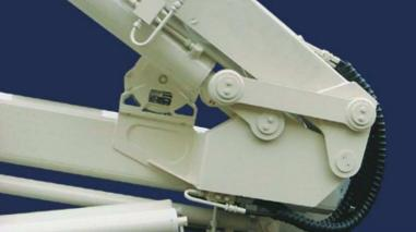
The link system of the outer boom gives additional power.
