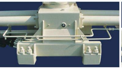
A heavy duty slewing system gives the capacity to operate the crane at max 7 degrees of heel without restriction of lifting capacity.
