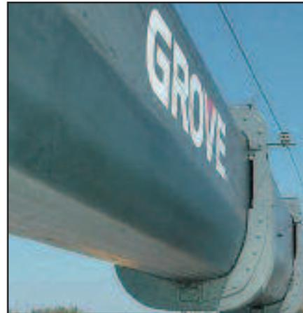
36 - 110 ft. (11 - 33.5 m) four section full power sequenced synchronized MEGAFORM™ boom designed for maximum vertical and lateral strength
