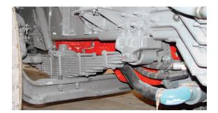
**Suspension** Spring front suspension with air ride rear suspension provides a comfortable ride at 105 km/h (65 mph).
