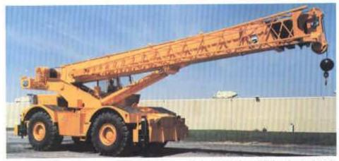
The "SwingAwey" lattice boom extension stows laterally along side the boombase section and swings easily into working position to provide 121 (36.9m) tip height with the standard boom and 147' (44.8m) up height with the optional boom.
