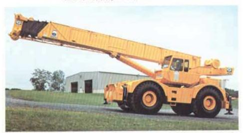
In addition to excellent mobility on all types of terrain, the HT75S leatures towoverall height, low center of gravity, excellent ground clearance and a GVW of approximately 74,000 bs. (33 566kg)
