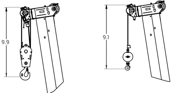
Dimensions are for the largest Grove furnished hook block and overhaul ball, with anti-two block activated.
