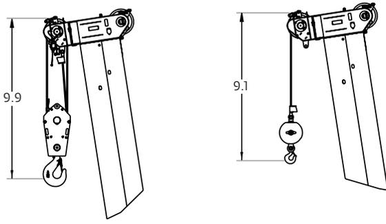
Dimensions are for the largest Grove furnished hook block and overhaul ball, with anti-two block activated.
