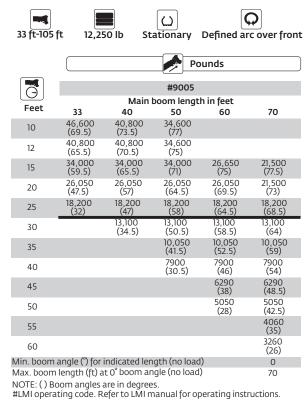
Lifting capacities at zero degree boom angle
