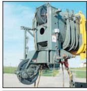
The RT700E has a quick-reeve boom nose and swingaway alignment device to help operators set up smoothly.
