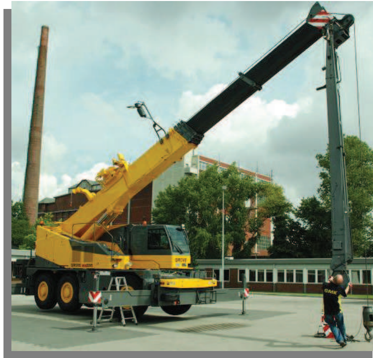
Twisting of the jib for bolting in.
