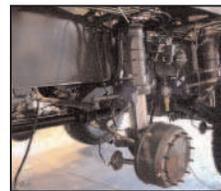
The exclusive Grove MEGATRAK™ independent suspension system allows all wheels to be on the ground at all times; now with top steering on rear axles.
