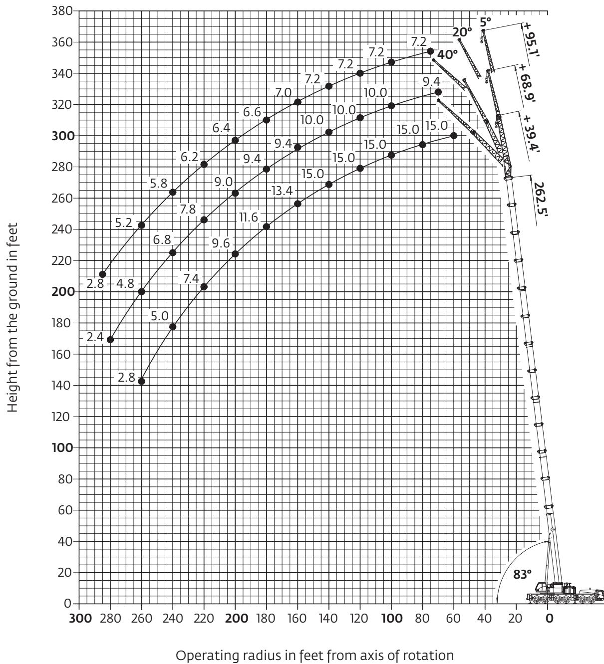
*Hook heights shown in the working diagram do not consider loaded boom deflection.*
