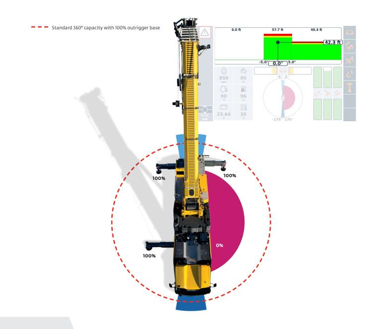
Obstacles on construction sites may prevent an outrigger from being extended. These are situations in which crane operators always had to accept reduced lifting capacities in the past because of a fully retracted outrigger base. MAXbase provides calculated charts for these instances where the crane can still use its full potential in some sectors. MAXbase also takes into account rear stability avoiding the crane to tilt backwards.
