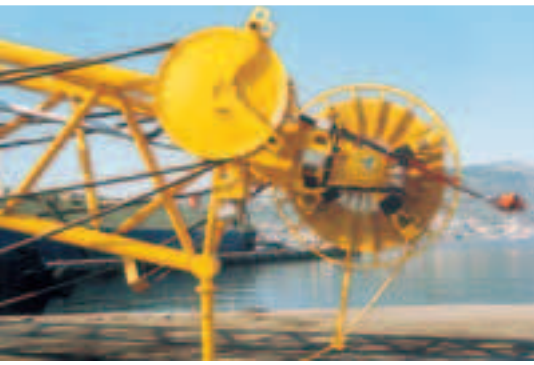
Cable reel on the boom head
