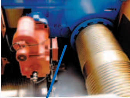
Hoisting gear with DC motor, spur gear and rope drum
