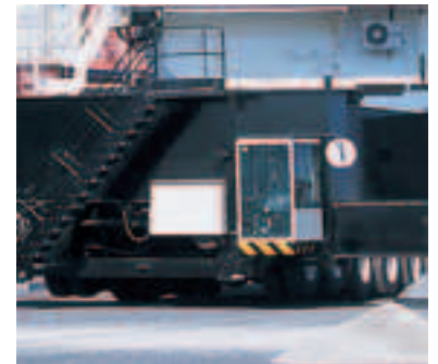
Additional cab on the chassis
