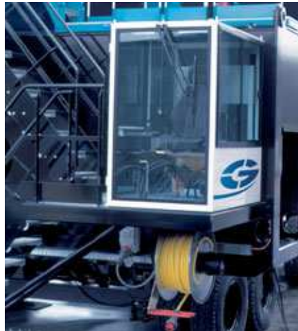
Additional cab on the chassis
