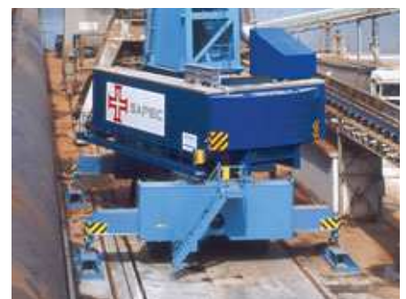
HMK 170 EG handling fertilizer at Sapec, Portugal: the field-tested H-shaped stabiliser arrangement enables the crane to operate even in areas with a minimum of working space
