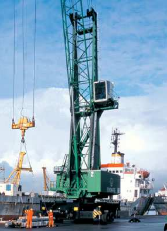
HMK 170 E handling general cargo at Zuidnatie at the Port of Antwerp, Belgium
