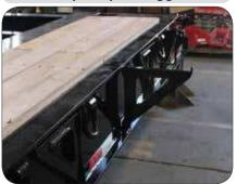
Standard heavy duty outriggers that span the entire height of the side rail allow for maximum force to be applied when in use.
