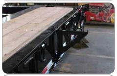
Standard heavy duty outriggers that span the entire height of the side rail allow for maximum force to be applied when in use.
