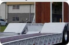
The 30 degree transition allows easier loading to the rear deck for equipment with lower ground clearance.
