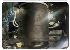
30,000 pound rated large diameter air bags are standard. This allows for lower operating pressure and higher capacity when needed.
