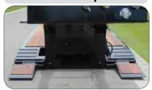
Adjustable wood filled ramps for varying load widths.
