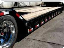
With a standard deck height of 24", Globe Trailers have lower overall height, which allows taller loads to be hauled.
