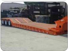
Bottom tapered beams allow for a lower load angle which will help to accommodate the loading of low angle pavers.
