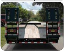
Adjustable with spring assist and safety bar.
