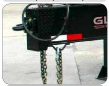
3" Pintle eye, with 4 adjustable height positions, with 2 heavy duty safety chains and grab hooks.
