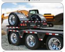
Globe Trailers has a patent on the hydraulic flip axle design. It allows for less down time when operating the flip axle and it can be easily detached when required.
