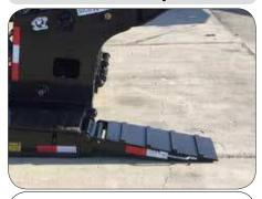
Low angle paver ramps for easy loading onto the main deck.
