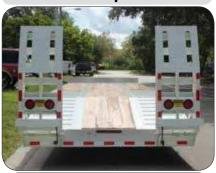
Adjustable with spring assist and safety bar.
