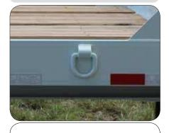
D-rings on each side of the deck make it easier to secure loads to the trailer.
