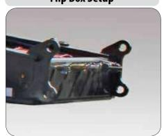
Flip box length options are available to achieve longer swing clearances when needed for longer truck frames or when coupling to single or multi-axle jeeps.
