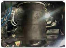
30,000 pound rated large diameter air bags are standard. This allows for lower operating pressure and higher capacity when needed.
