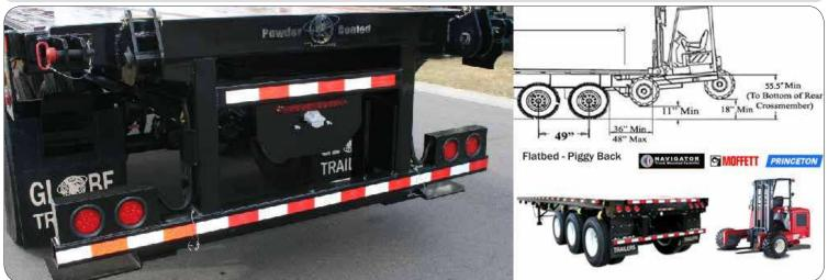
Optional Piggy Back setup for forklift mounting. Universal for Moffett, Princeton and Navigator forklifts.
