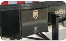
Optional Lockable Tool Box Mounted Underside of Main Deck, 24" x 24" x 48" Steel, can be located on either side.
