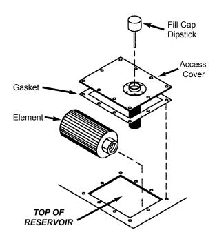
Hydraulic Reservoir Sump Strainer Removal
