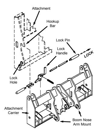
**Attachment Release Mechanism**
