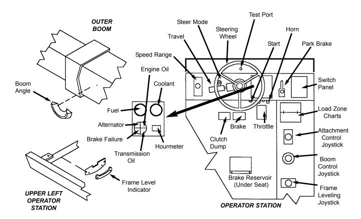
**Operator Compartment & Boom Indicators/Controls Location**
