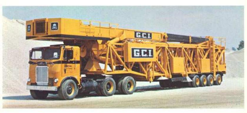
The 5400 is a completely mobile self-erecting hydraulic crane. In tractor trailer configuration it travels at a highway speed of 50 mph. The 40' jib, blocks and all rigging are mounted on the crane. Once outriggers are set, the main mast erects hydraulically from horizontal to vertical position and telescopes to operational height in minutes.
